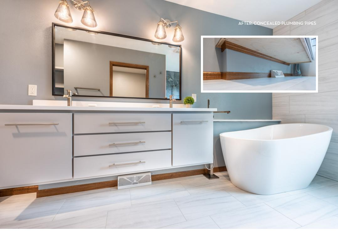
Again, we came up with another solution, to build a small wall around the plumbing pipes. This would give the illusion of a floating vanity, conceal the plumbing pipes below, as well as offer a foundation for the vanity to support itself on - still floating, yet very well supported!
